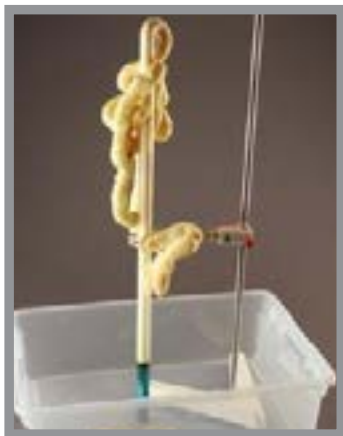
Tube of Toothpaste Demonstration (Catalytic Decomposition of Hydrogen Peroxide) Ward's Item Number 2005600
